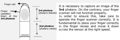
A finger scanner works like a camera. It makes a picture of the bottom side, the papillary lines, of vour finger's third phalanx. However, this picture must be of good quality, so that physical access can be granted whenever necessary
