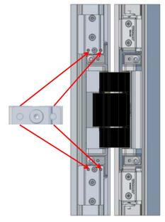
Screw or unscrew the 4 screws. 2 right and 2 left, adjustment range +/- 1mm.
