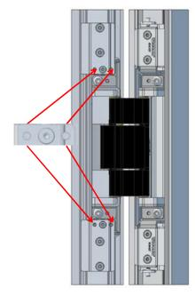
Loosen the screws for the top and bottom hinges
