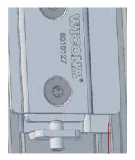
Turn screw with ball end on top and bottom hinge for adjustment, range +/- 3mm
