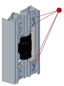
Tighten screws on top and bottom hinges, torque 15Nm.
