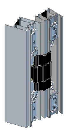
Tighten the 4 fixings screws 6 torque 15Nm.
