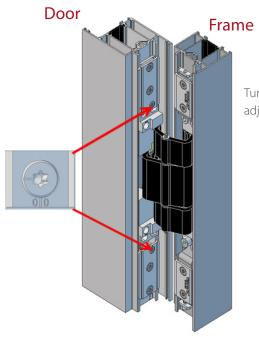
Turn the central screws (T25) to adjust horiziontally, +/- 2mm
