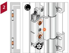
To minimise the shadow groove please tighten the clamp screws.
