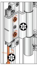
Tighten clamp screws of the door hinge blades and bring the set screw into position.
