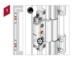
Loosen adjustment screws.
