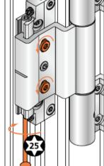
Loosen the clamp screws of the door hinge blades on all hinges, loosen bottom set screws (approx. 3 turns).
