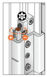
Adjust the height  $\pm$  3 mm by using the upper set screw.
