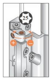
Adjust the height  $\pm$  3 mm by using the upper set screw. Important: The lower hinge supports the door.
