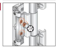
Tighten adjustment screws (4 – 6 Nm).
