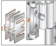
Remove spacer plates (3 x 0.5 mm).
