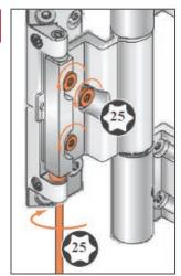
Loosen the adjustment screws on the door hinge blades on all hinges, loosen bottom set screws (approx. 3 turns)
