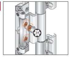
Loosen adjustment screws.
