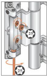
Tighten adjustment screws on the door hinge blades and bring the set screw into position.
