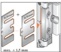
Combine the required number of spacer plates (each 0.5 mm) Adjustment of  $\pm$  1.5 mm possible in 0.5 mm increments.
