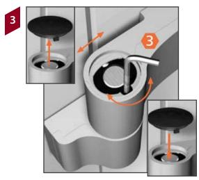
Remove cap. Adjust horizontally by turning the spindle on the upper hinge section (± 2.5 mm).
