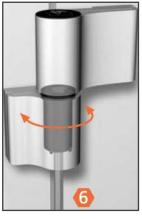
Turn the bearing bushing  $\pm$  90° until you feel it catch (sealing pressure  $\pm$  0,5 mm)
