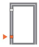
Carry out height adjustment only on bottom hinge. Re-adjust only upper hinges.
