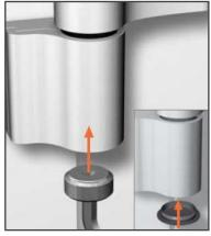
Screw lifting and lowering spindle back in. Snap on cap.
